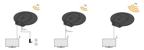
Intelligent TV antenna with BOSS system (Balanced Output Signal System) that adjusts in real time to always offer the best TV signal automatically.
