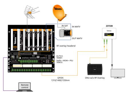
Due to its characteristics, its usefulness as a complement to ONT/ONU modules without RF output.
