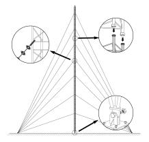
It consists in fixing the lower section to the base, set it in upright position and levelling it. The subsequent Middle Sections are then mounted, equipped with the appropriate guy wires; the mounting is carried out by climbing on the previously mounted sections and hoisting the new section with the help of the appropriate lifting tools.
