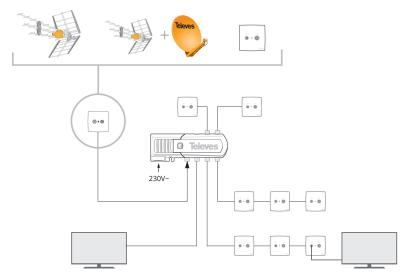
Connector type and number of outputs according to reference
