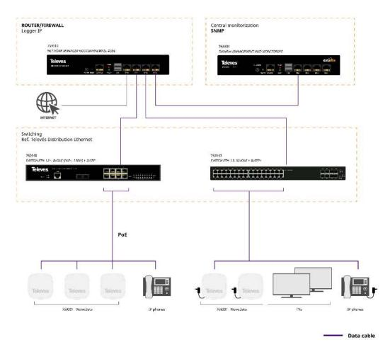
GPON installation: FTTR architecture that provides Quadruple play services (TV, Telephone, Data and WiFi) to the rooms.
