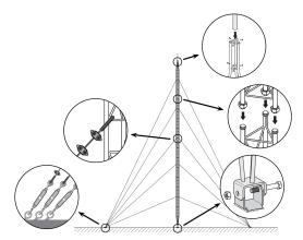
It consists in fixing the lower section to the base, set it in upright position and levelling it. The subsequent Middle Sections are then mounted, equipped with the appropriate guy wires; the mounting is carried out by climbing on the previously mounted sections and hoisting the new section with the help of the appropriate lifting tools.
