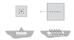
Turret base foundation ground plate (Central node) and guy wires foundation ground plates (intermediate/external node).
