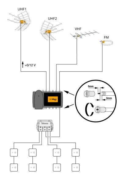
NOTE: To avoid damaging the amplifier, we strongly recommend switching OFF the amplifier until the installation process has been completed.
