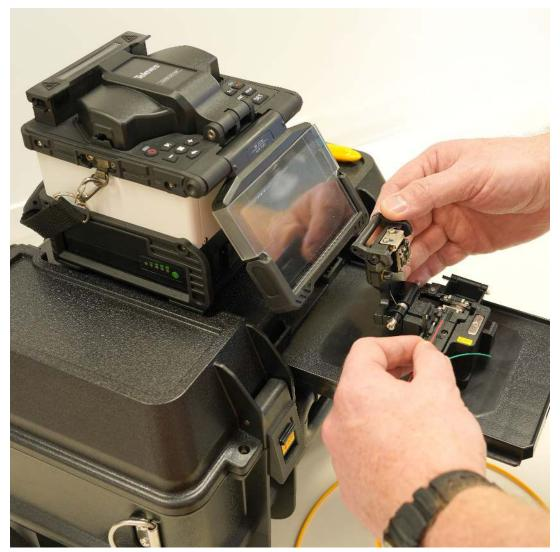
The integrated tray in the case is able to support the fusion splicer, providing an uncluttered and agile working area. We recommend adding weight to the inside of the case to ensure stability during use.
