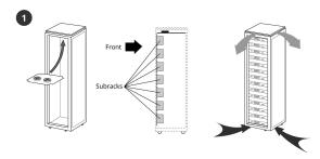
Fans are located in a screwed tray at the top of the
