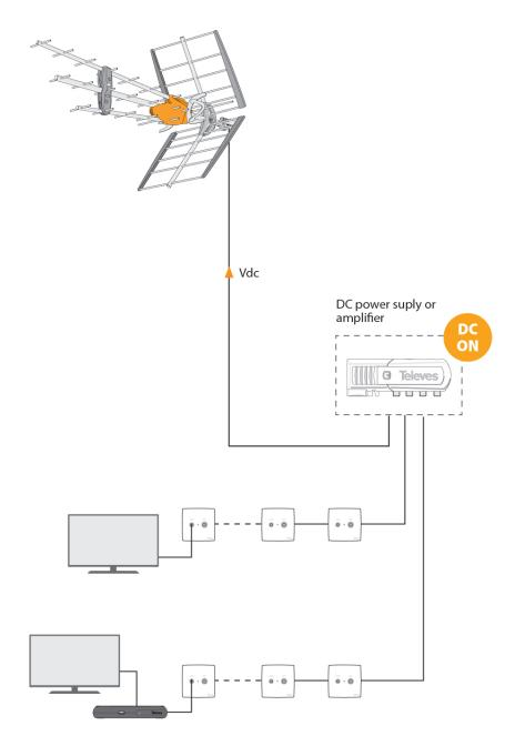
BOSS activation by means of a power supply unit or an amplifier.
