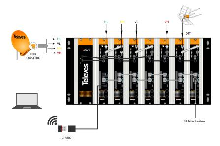
This adapter must be connected to the micro USB port on the front of the unit. After an automatic initialization process, connection to a Wi-Fi network will be possible, provided its SSID has the following format: Televes\_mng\_XXYYZZ. To go to the configuration website, open a browser and go to the URL "config.t0x".
