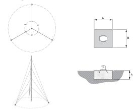
Turret base foundation ground plate (Central node) and guy wires foundation ground plates (intermediate/external node).
