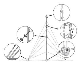
It consists in fixing the lower section to the base, set it in upright position and levelling it. The subsequent Middle Sections are then mounted, equipped with the appropriate guy wires; the mounting is carried out by climbing on the previously mounted sections and hoisting the new section with the help of the appropriate lifting tools.
