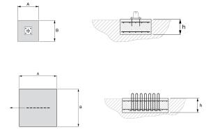
Turret base foundation ground plate (Central node) and guy wires foundation ground plates (intermediate/external node).
